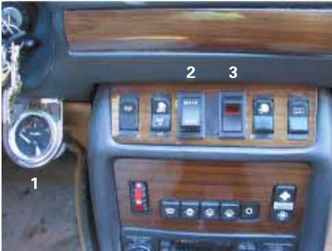
1) the auxiliary veggie fuel gauge, 2) fuel-type switch, and 3) back-flush switch on the dash of the 300CD.
