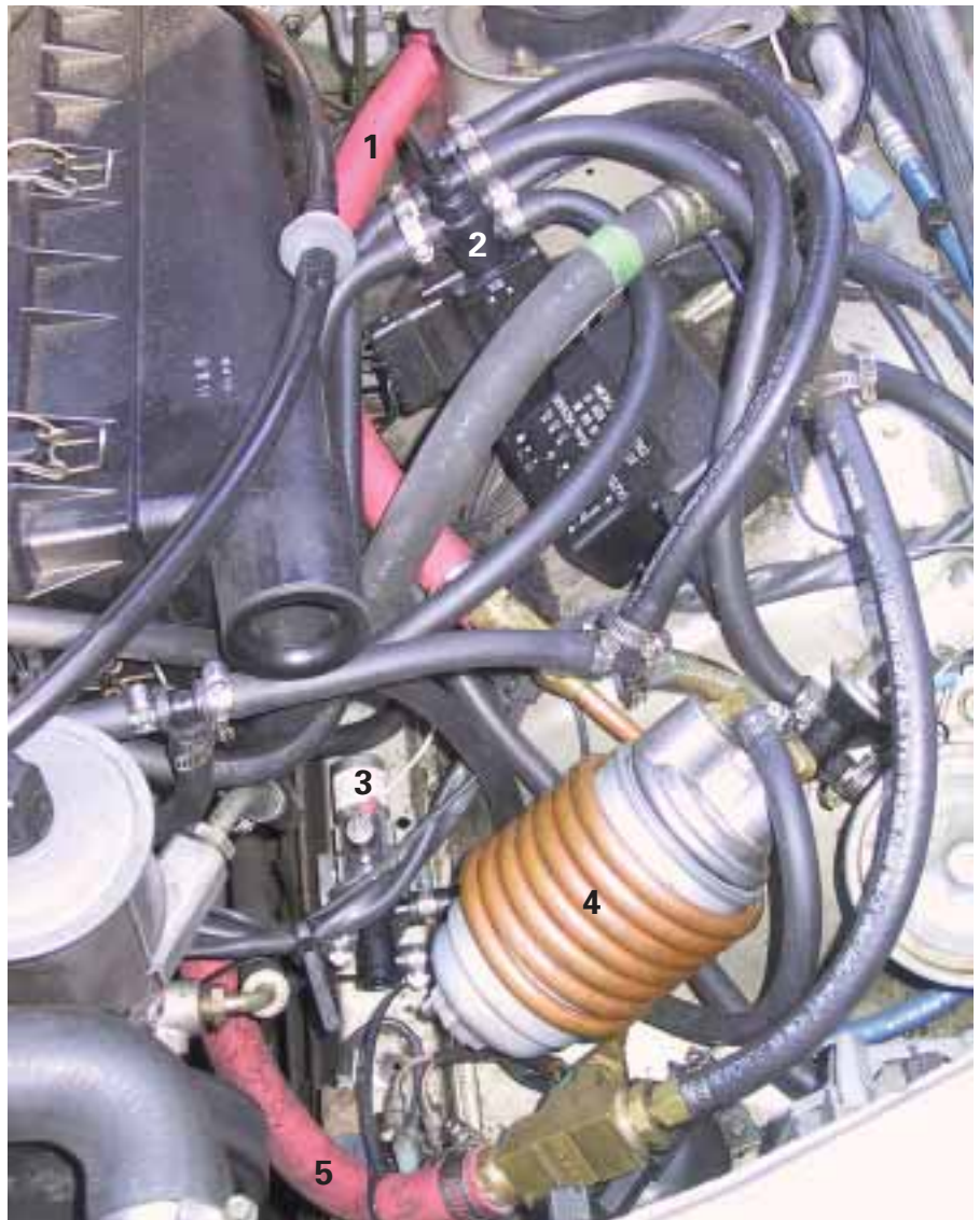
Under the 300CD's hood: 1) heater hose from heater-core splice; 2) six-port solenoid fuel switch; 3) three-port solenoid fuel switch; 4) vegetable oil heated filter; 5) HIH back to/from vegetable oil tank.
