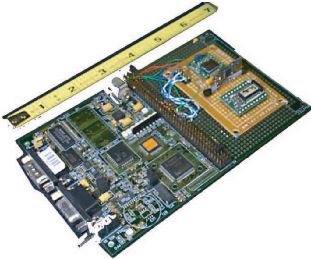
Fig. 4. A close-up of the low-cost attitude solution used on the Atlantis, and pictured in Fig. 3. The ruler is there for scale, and shows that the entire board is less than 6 inches long and 4 inches across. The microcontroller is an Infineon 515 processor, and the attitude is being relayed on the CAN bus.
