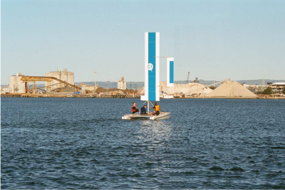
Fig. 1. The Atlantis, based on a Prindle-19 Catamaran, with a self-trimming wingsail. The Atlantis was designed to demonstrate a very high precision of navigation and control, even in the presence of wind and waves. As shown here, testing in Redwood City harbor, January 2001, the Atlantis was able to achieve line following to better than 30 cm. 1 - \sigma under wind propulsion. The author and colleagues on board are human ballast to prevent capsizing during this initial test.
